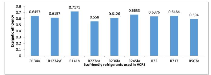
Figure 18: Thermal second law performances(Exergetic Efficiency \_VCRS) of cascade single effect LiBr vapour absorption refrigeration system coupled with vapour compression refrigeration using ecofriendly refrigerants in the low temperature cycle of VCRS system
