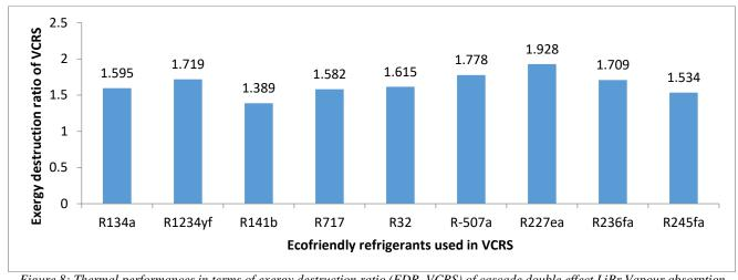
Figure 8: Thermal performances in terms of exergy destruction ratio (EDR\_VCRS) of cascade double effect LiBr Vapour absorption refrigeration system coupled with vapour compression refrigeration using ecofriendly refrigerants in the low temperature cycle of VCRS system
