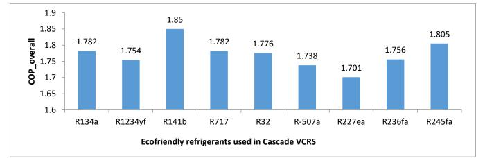
Figure 1: Thermal first law performances (COP\_Over all) of cascade triple effect LiBr vapour absorption refrigeration system coupled with vapour compression refrigeration using ecofriendly refrigerants in the low temperature cycle of VCRS system
