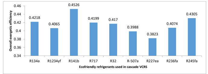
Figure 3: Thermal second law performances (Overall Exergetic Efficiency) of Cascade triple Effect LiBr vapour absorption refrigeration system coupled with vapour compression refrigeration using ecofriendly refrigerants in the low temperature cycle of VCRS system
