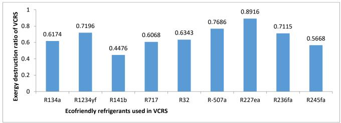
Figure 11: Thermal performances in terms of exergy destruction ratio (EDR\_VCRS) of cascade double effect LIBr vapour absorption refrigeration system coupled with vapour compression refrigeration using ecofriendly refrigerants in the low temperature cycle of VCRS system
