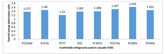
Figure 2: Thermal performances in terms of exergy destruction ratio (EDR\_VCRS) of cascade triple effect LiBr vapour absorption refrigeration system coupled with vapour compression refrigeration using ecofriendly refrigerants in the low temperature cycle of VCRS system
