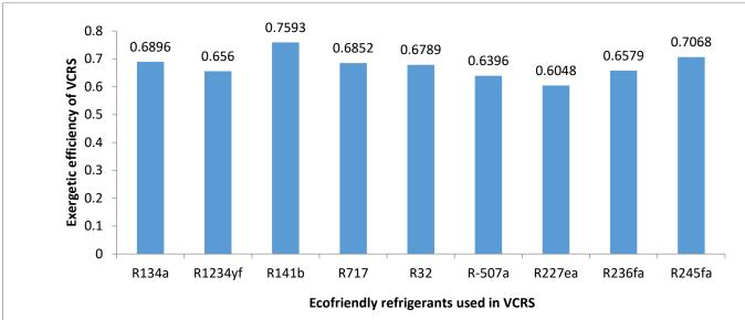
Figure 6: The exergetic efficiency of vapour compression of refrigeration system coupled with vapour compression refrigeration using ecofriendly refrigerants in the low temperature cycle of VCRS system
