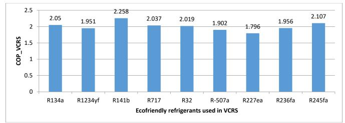
Figure 4: Thermal first law performances (COP\_VCRS) of cascade triple effect LiBr vapour absorption refrigeration system coupled with vapour compression refrigeration using ecofriendly refrigerants in the low temperature cycle of VCRS system
