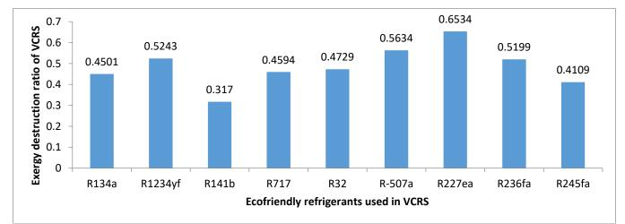
Figure 5: Thermal performances in terms of exergy destruction ratio(EDR\_VCRS) of cascade triple effect LiBr vapour absorption refrigeration system coupled with vapour compression refrigeration using ecofriendly refrigerants in the low temperature cycle of VCRS system
