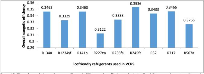
Figure 15: Thermal second law performances (Exergetic Efficiency\_Overall) of cascade single effect LiBr vapour absorption refrigeration system coupled with vapour compression refrigeration using ecofriendly refrigerants in the low temperature cycle of VCRS system
