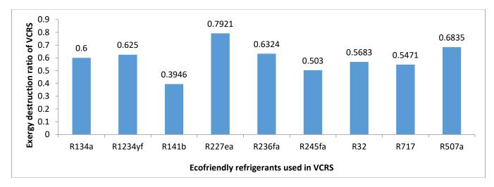
Figure 17: Thermal performances in terms of exergy destruction ratio (EDR\_VCRS) of cascade single effect LiBr vapour absorption refrigeration system coupled with vapour compression refrigeration using ecofriendly refrigerants in the low temperature cycle of VCRS system
