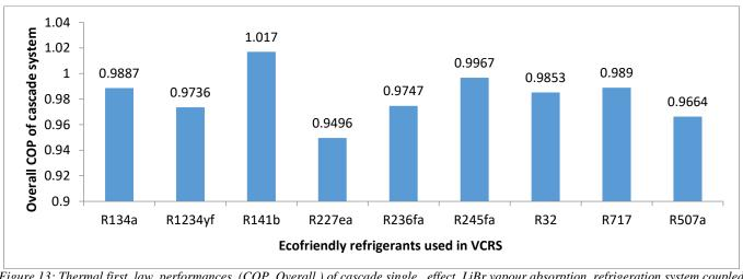
Figure 13: Thermal first law performances (COP\_Overall) of cascade single effect LiBr vapour absorption refrigeration system coupled with vapour compression refrigeration using ecofriendly refrigerants in the low temperature cycle of VCRS system
